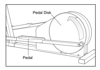
To dismount the elliptical, allow the pedals to come to a complete stop. **CAUTION:** The elliptical does not have a freewheel; the pedals will continue to move until the flywheel stops. When the pedals are stationary, step off the highest pedal first. Then, step off the lowest pedal.
